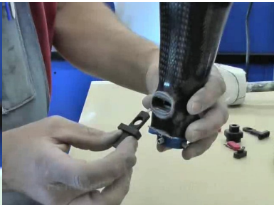
33. Slide lock plate into face plate and install spring.
