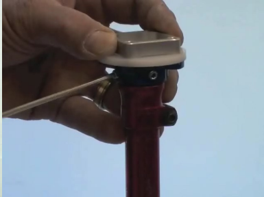
21. Attach pyramid to endo components. All components should be at neutral. Return mold and lock to alignment fixture.
