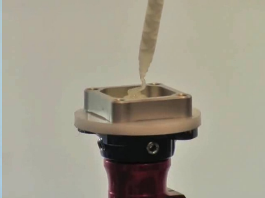
22. Check height measurement to ensure height is identical to test socket. Fill connector with glue.
