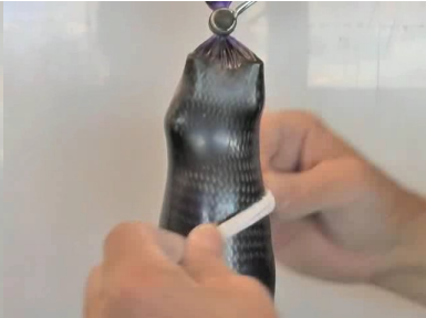
29. Pull outer PVA bag over mold. Laminate in customary fashion.
