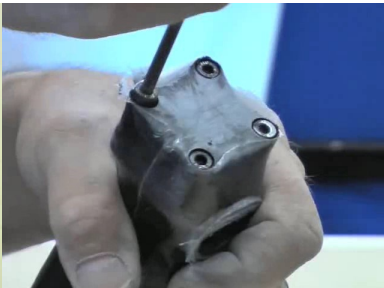
32. Remove Eight Hole Plate. Finish socket as usual.
