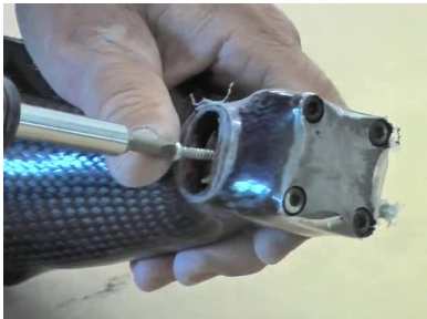
31. Remove foam rectangle and red silicone caps. Install removal screw in lamination tool. Remove lamination
