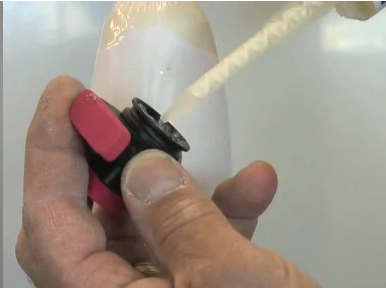
18. Apply a bead of glue to housing funnel and glue to anchor with lamination tool aligned with release button location mark.
