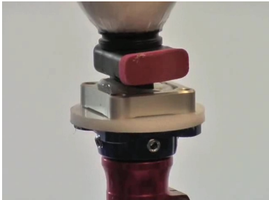
23. Lower mold and lock onto connector. Allow glue to set.
