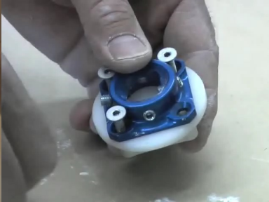
20. Place glue plate on connector. Install pyramid to connector. Do not over tighten screws.
