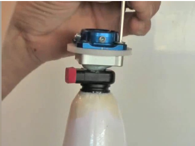
25. Remove screws from connector.
