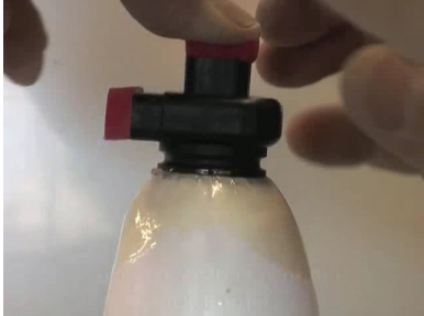
19. Ensure PVA bag is under lock funnel
