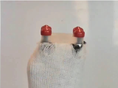
28. Lube attachment screws. Install Eight Hole Plate. Do not over tighten screws. Install red silicone caps onto screws. Finish Layup
