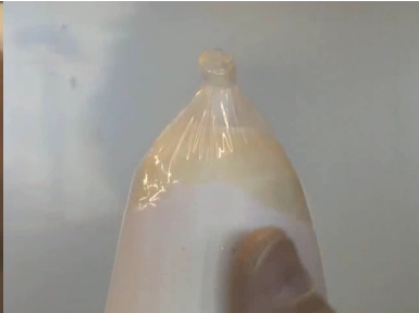
17. Pull PVA bag over cast. Use heat to help ensure PVA fits under lock funnel.
