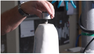
Put CD103FD fabrication dummy over anchor.
