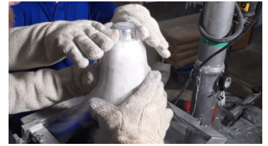
Pressing in around fabrication dummy will help remove any air pockets.
