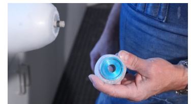
Remove tooling from anchor.
