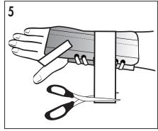
5. Ensure Fit Knuckles should not be obstructed, and brace should fit snug. Trim straps if necessary.
