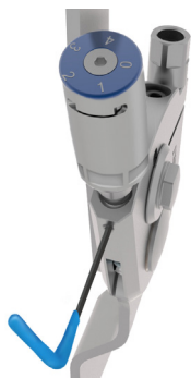
Figure 1. Unlock / lock the PF ROM Adjustment using the 1.5mm hex wrench to loosen / tighten the ROM Lock Set Screw.
