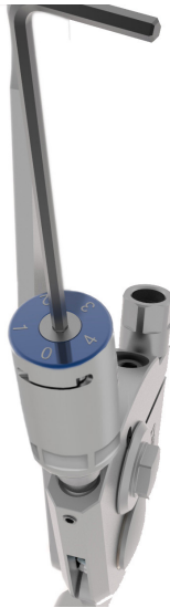
Figure 5. Remove the ROM Dial Screw and PF ROM dial.
