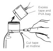
10. Wrap one layer of vinyl tape over the remaining half-width of tape to completely seal the cast from resin leakage.
