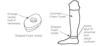
Note: Cut the foam cosmetic cover 1" or 25 mm longer than necessary so that the compression of the foam cover will hold the Shaped Foam Ankle securely against the Impulse foot.
