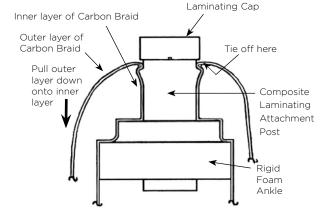
23. Reinforce the layup with carbon tape applied from the original lamination to the tie-off groove and back up to the original lamination, as shown at right. Apply additional reinforcement if required. Proceed with the lamination, using standard procedures.
